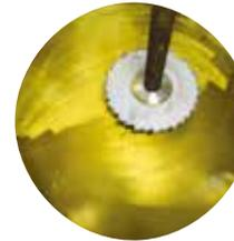
The desired image is impressed on the barrel by applying paint on a personalized screen that touches the barrel while it rotates. The personalized barrel is left to rest for at least 4/6 hours, to avoid any damage in the next steps of the production.
