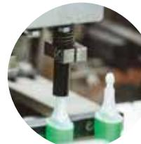
This process involves the assembly of the felt pen, by combining together the plastic components, the filter, the ink and the nib. The process is completely automated. After the various stages of assembly, the ink will move from the filter to the nib through a capillary effect; the nib will release the ink gradually while writing.
